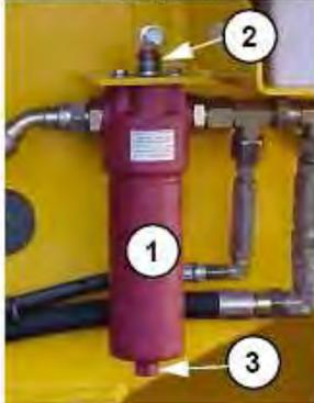
Photo 16 Travel circuit hydraulic oil filter
